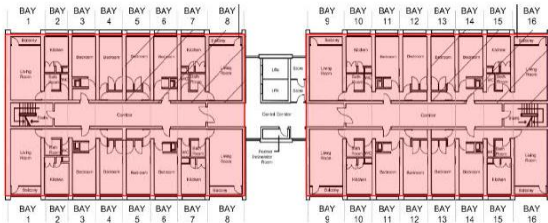
Figure 2.2 – Typical St James House floor layout showing areas where strengthening is required
